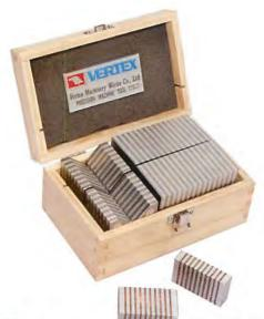
Non-magnetic laminated plates and blocks are extras to increase the versatility of chucks. These plates and blocks offer excellent guidance of the magnetic force, and can be used in combination with chucks as 'extensions' for the clamping of workpieces of complex shapes.
