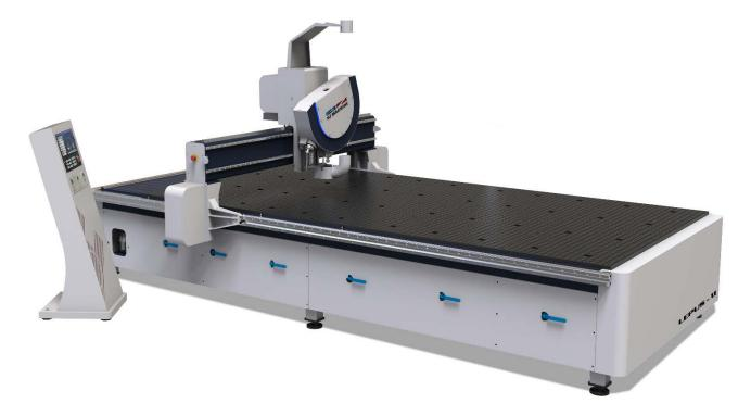
The 3-Axis CNC controlled panel processing machine LEPUS - II and II L is intended for cutting, v-channel opening and similar operations on various composite panels and plates.
