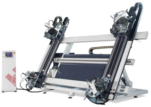
APEX - IV features simultaneous assembling of all 4 corners of the profile by combining the precision of servo measuring and power of hydraulic system to offer quick solutions to users.
