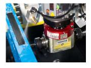
By focusing on providing convenient solutions for customers, and combining power and precision, GARNET XS lets the processing capacity be only limited by the users imagination, thanks to the 5.5 kW spindle motor with automatic tool replacement feature.
