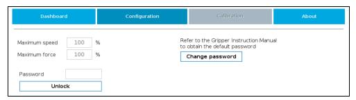
Fig. 4-12: Limiting the Gripper Force and Speed
