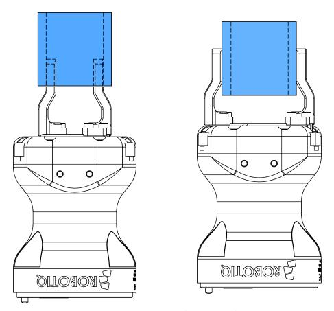
Fig. 1-4: Hand-E gripper internal and external gripping.
