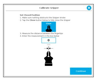
Fig. 4-16: First step of the calibration wizard
