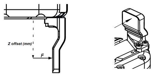
Fig. 5-10: Z-axis offset at which force/payload is applied.
