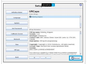
Restart PolyScope to complete the URCap installation. By doing so, you
