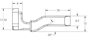
Fig. 5-6: Flat NBR overmolded finger.
