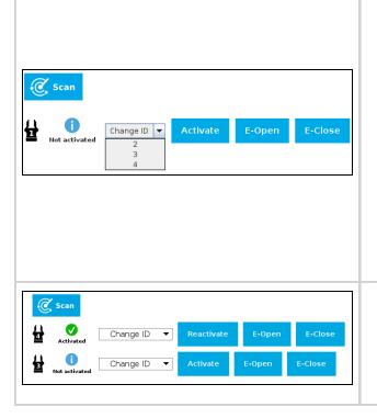
Check that gripper ID is different from that of other grippers that will be connected to the robot, and if required, select a different ID from the "Change ID" dropdown list.
