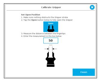
Fig. 4-17: Second step of the calibration wizard
