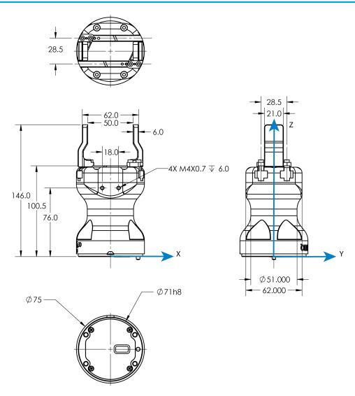
Fig. 5-1: General dimensions of Hand-E (open).
