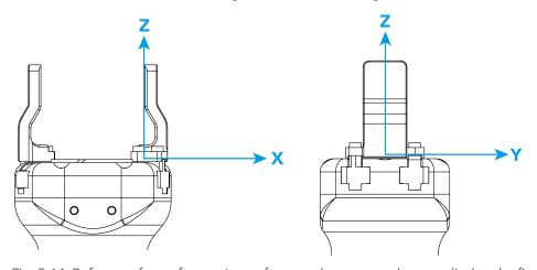
Fig. 5-14: Reference frame for maximum force and moment values applied to the fingers
