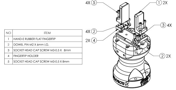
Fig. 3-8: Mounting fingertips on holders, and holders on racks.
