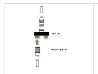
1. Connect only one gripper at a time using the splitter.
