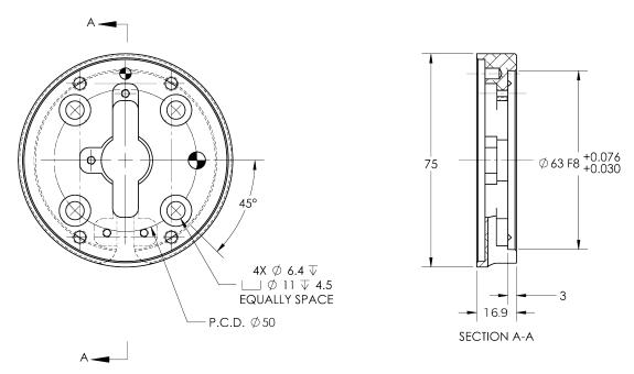
Fig. 5-3: Coupling for ISO 9409-1-50-4-M6.
