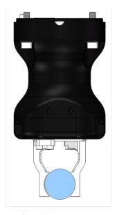
Fig. 5-12: Friction grasp and form-fit grasp.
