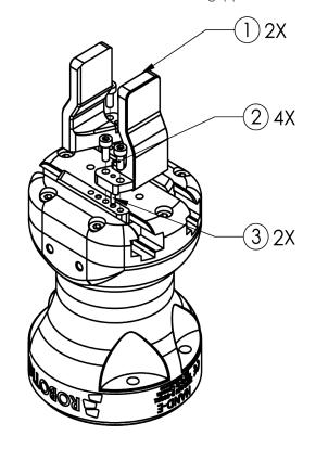
Fig. 3-7: Mounting fingers on racks.
