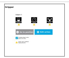
When the node is not defined, the Command window shows warning messages. Tap **Edit action** to modify the Gripper's action.
