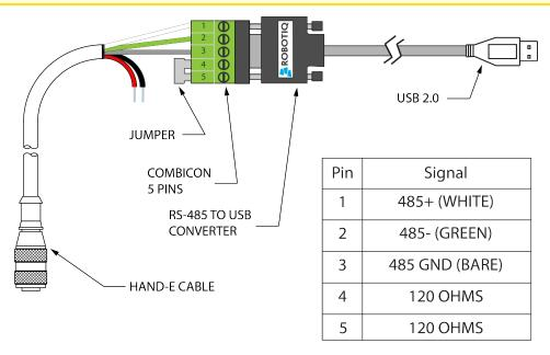
\*24 V AND GND ARE NOT SUPPLIED VIA USB \*120 Ohms resistance JUMPER BETWEEN PINS 4 AND 5
