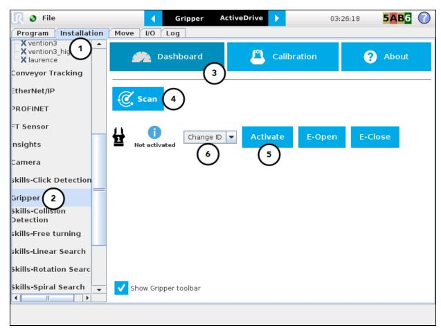
Fig. 4-10: Gripper Dashboard (steps highlighted)
