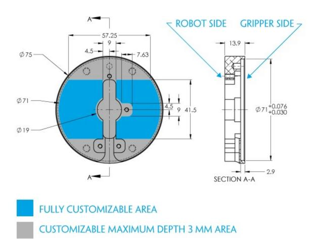
Fig. 5-2: Workable area dimensions of blank coupling AGC-CPL-BLANK-002
