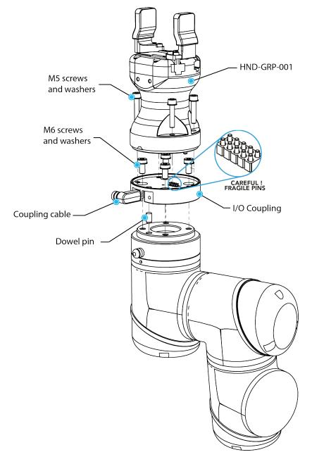
Fig. 3-4: Mechanical installation of the I/O Coupling and the Hand-E gripper
