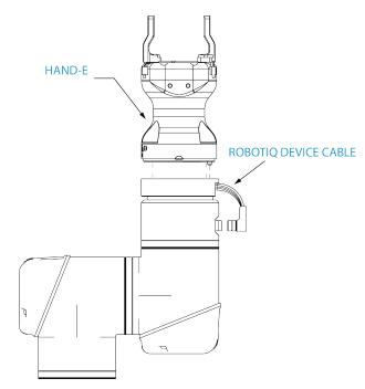
Fig. 3-10: Robotiq Hand-E with device cable wiring scheme
