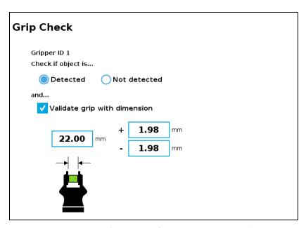
Fig. 4-28: Grip Check node interface with dimension validation
