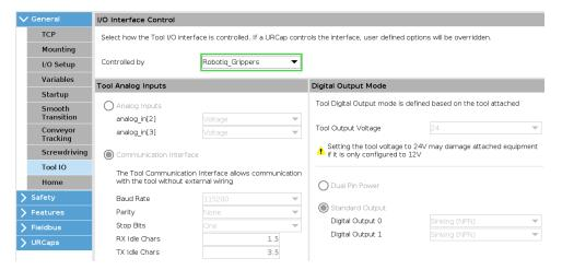
Fig. 3-14: I/O Interface Control.
