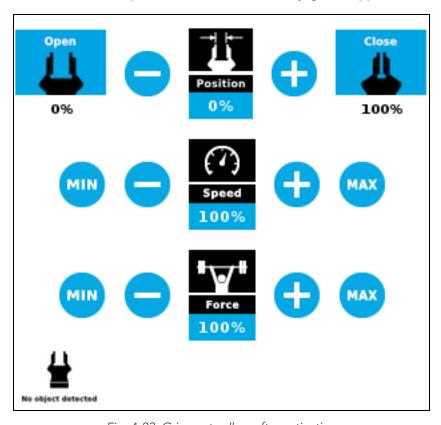
Fig. 4-23: Gripper toolbar after activation
