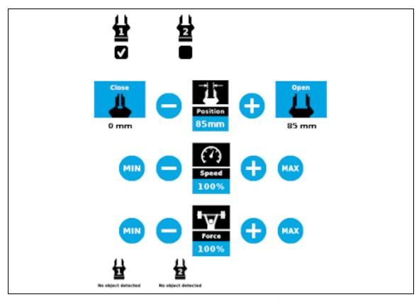
Fig. 4-24: Gripper toolbar (expanded, multiple Grippers)
