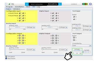
Fig. 8-3: Voltage set to 24V.
