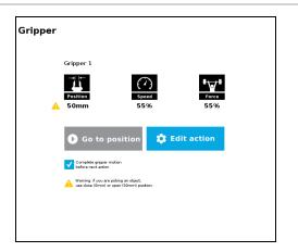
When the node requests the Gripper to close/open, the Command window warns that a partial opening/closing should not be performed for picking an object.
