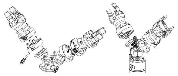
Fig. 3-5: Dual Hand-E Gripper Configuration (CB-Series and e-Series)
