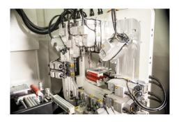
With its 13 fan cooled spindle motors, triple grip slot opening motor and saw blade motor ALCOR - II R can perform 15 different operations simultaneously and facilitates performance of operations without any limits on 4 different surfaces of the profile.
