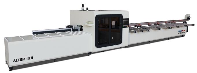
The 8-axis CNC profile machining and cutting center ALCOR - II R has been developed to carry out all-in-one cutting, milling, drain channel opening, punching and marking operations on PVC profiles. Thanks to its 14 machining and individually operating units, ALCOR - II R has been designed to offer maximum efficiency in less time.
